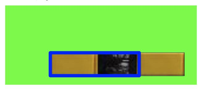
In the above image, the green represents the external noise in the camera position when autonomous is initialized. By cropping the above image to within the blue border (shown below), all the positions of the skystones can be determined.
